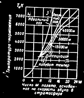
Fig. 9 - The temperature of retardation for bodies moving at different M_s and different altitudes.
