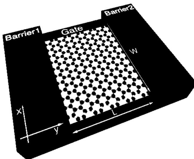
**Figure 2. Quantum dot in graphene nanoribbon. A ribbon of graphene with semi-conducting armchair boundaries is schematically shown. Two barrier gates (blue) define the rectangular size of the quantum dot (with width  $W$  and length  $L$ ). A back gate (red) allows one to shift the energy levels in the dot. Two or more quantum dots of this type can be easily put in series in a single nanoribbon.**
