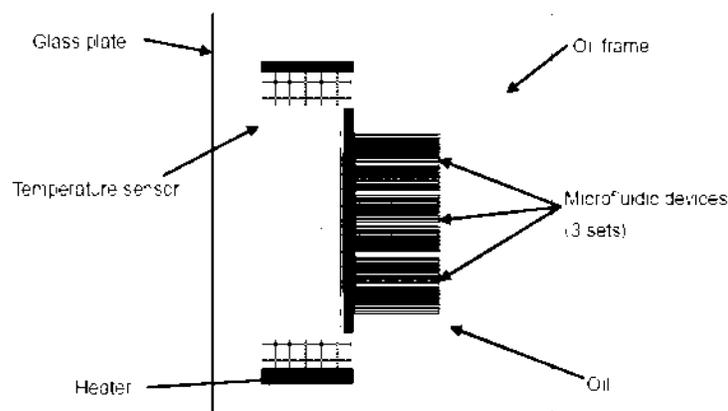
Figure 16. Micro-fluidic device for DNA tile self-assembly.
