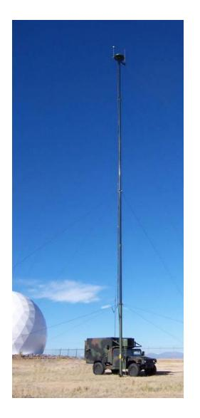
The Composite Tracking Network (CTN) system is a truck-portable radio antenna that allows line-ofsight connection to the Cooperative Engagement Capability (CEC).
