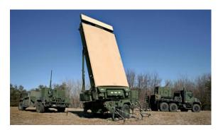
a common hardware baseline. The ability to define the radar's mission provides a long-term solution for air surveillance, air traffic control, counterbattery, and weapons control that is adaptable with technological developments. G/ATOR detects and tracks the most challenging indirect fire and low observable/low radar cross-section air threats at tactically significant ranges.
