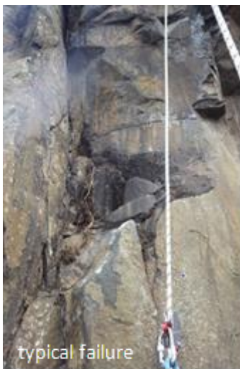
typical roots found behind rock failure
