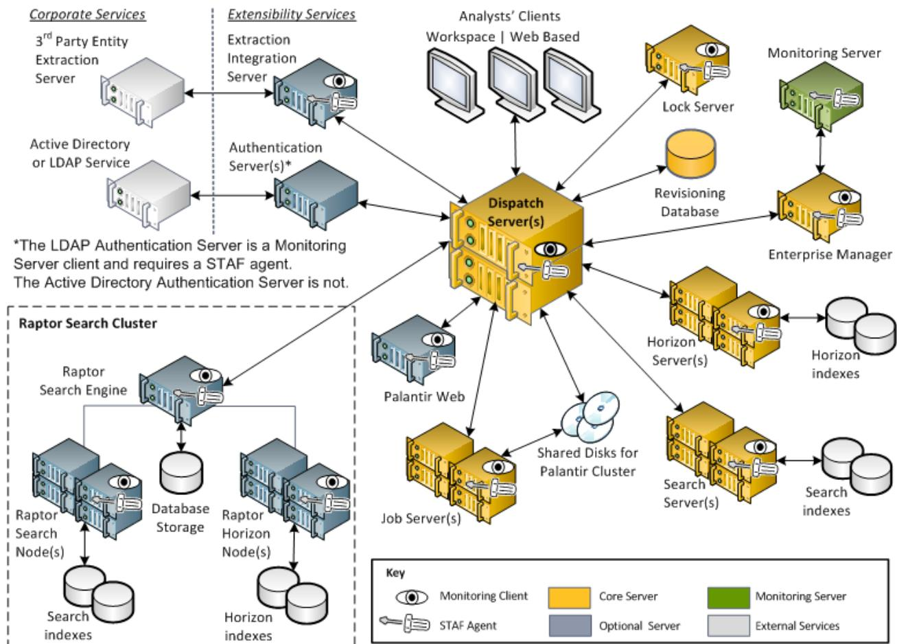
The Palantir core product servers can search and analyze data that has been imported into, or created in, Palantir. The core product consists of a Dispatch Server, a Job Server, a Search Server, a Horizon Server, and the Palantir Enterprise Manager.
