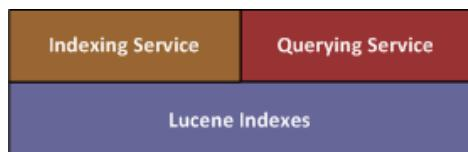
Palantir has heavily modified the Lucene implementation, adding the enterprise-level security and scaling characteristics of an enterprise-grade server. This server is integrated with the dynamic ontology, and it includes a number of customizations to the fuzzy-search capabilities of the information retrieval library.
