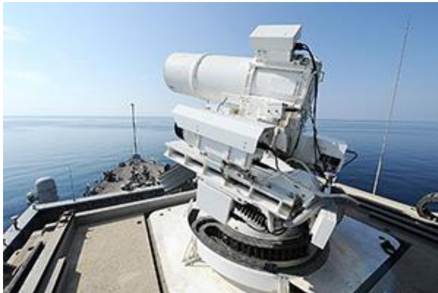
Figure 2. Laser Weapon System (LaWS) on USS Ponce
