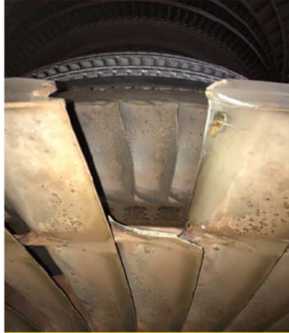
Figure 6. Missing turbine blade of L-1 section of LH. 20
