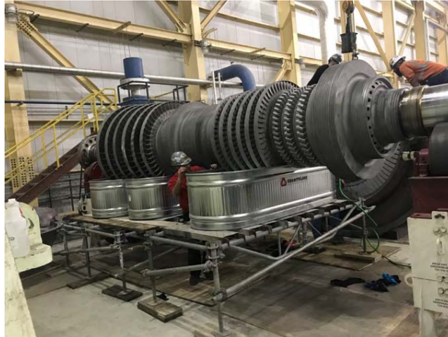
Figure 1. Comanche 3 high pressure, intermediate pressure (HP-IP) rotor.
