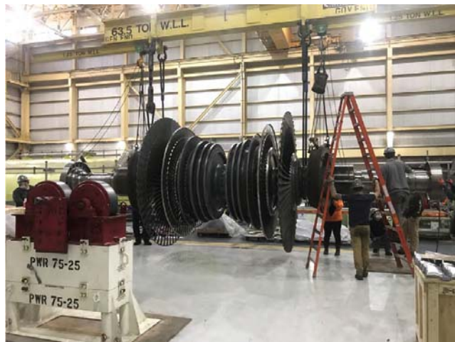
Figure 2. Comanche 3 low pressure A (LPA) rotor.
