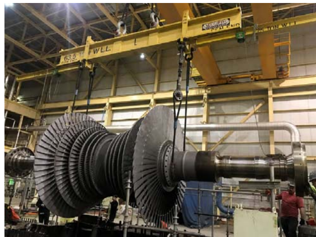
Figure 3. Comanche 3 low pressure B (LPB) rotor.
