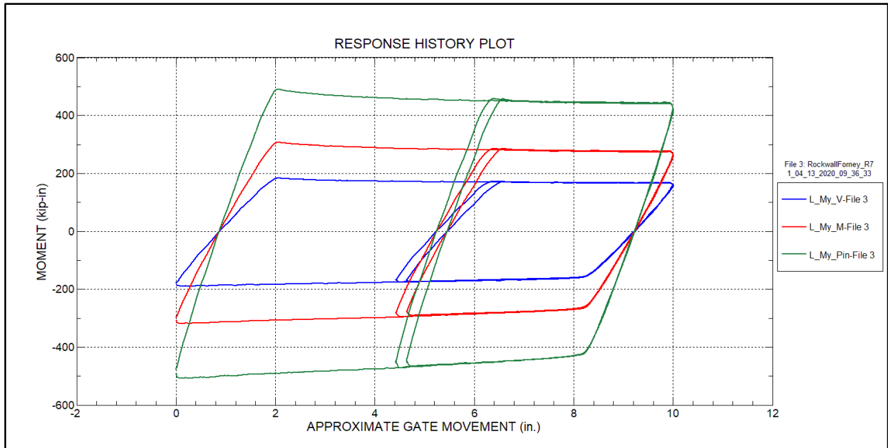
Figure 36 – Pin moment response history – Left arm – Test run 3
