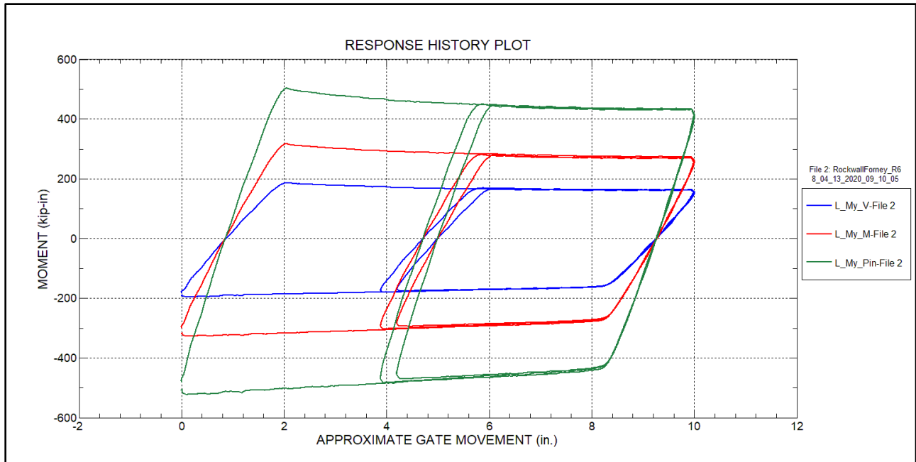
Figure 34 – Pin moment response history – Left arm – Test run 2
