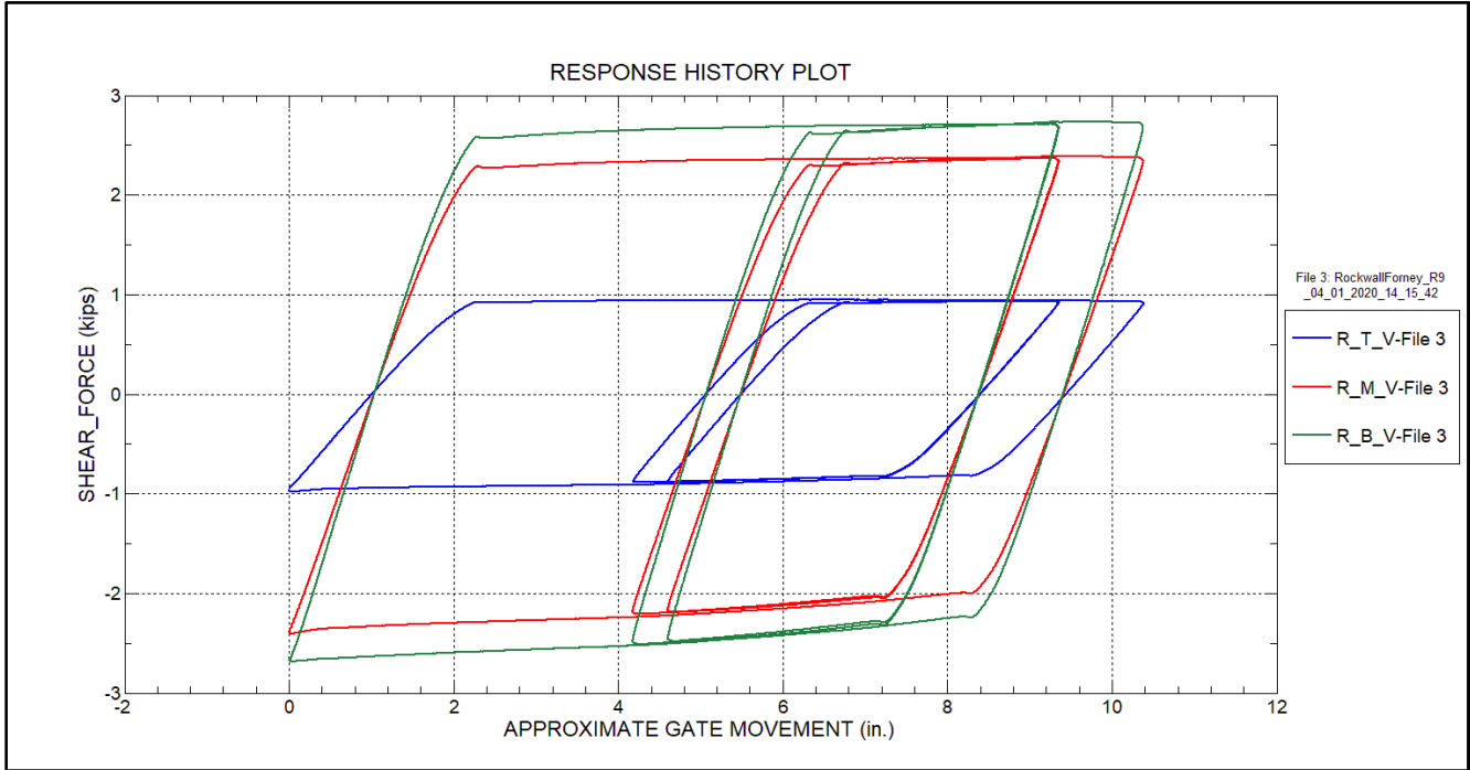
Figure 19 – Strut shear response history – Right arm
