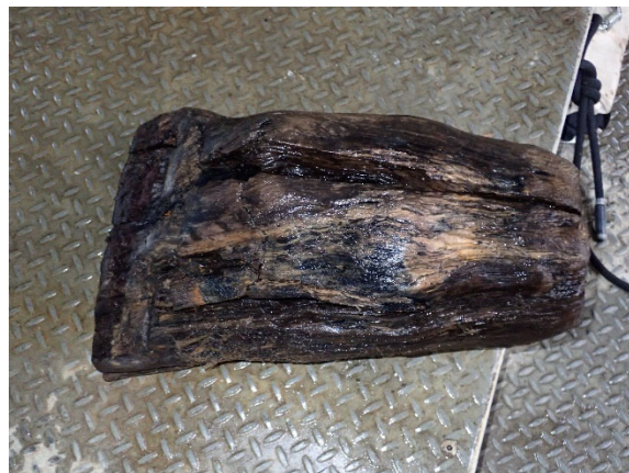
Photo 5-9: Log recovered from below the gate.
