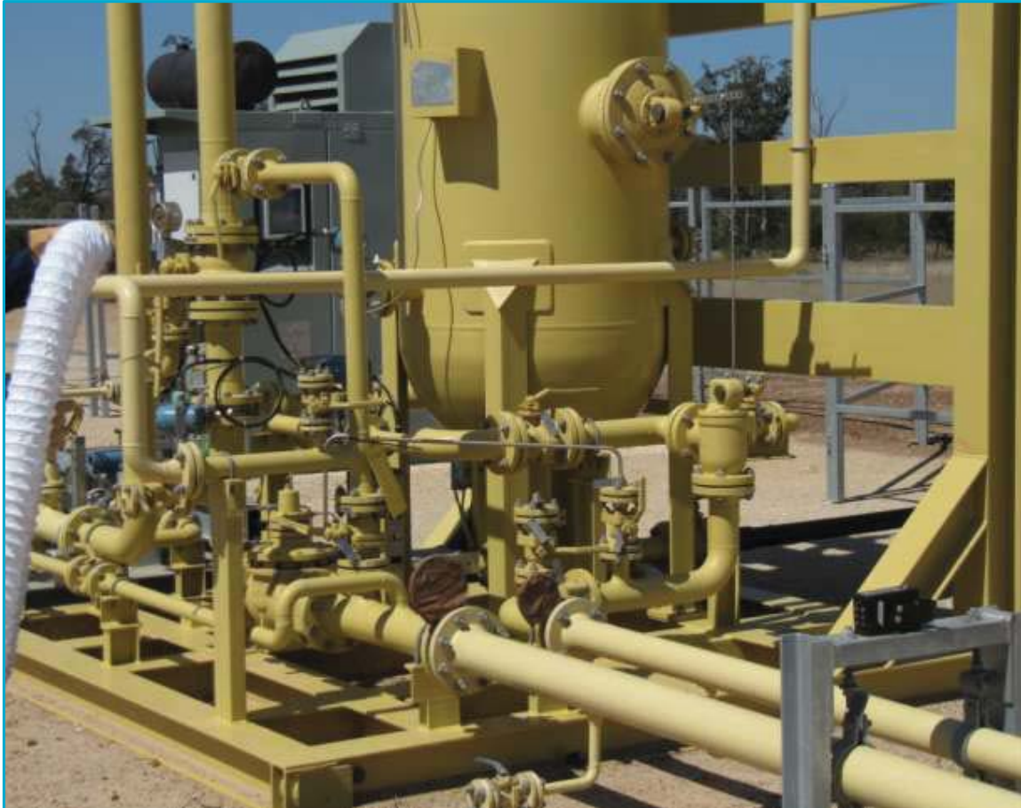
Figure 4.3. CSG well pad showing some of the surface equipment and potential emission points. Note the engine in the background for supplying hydraulic power to the water pump.
