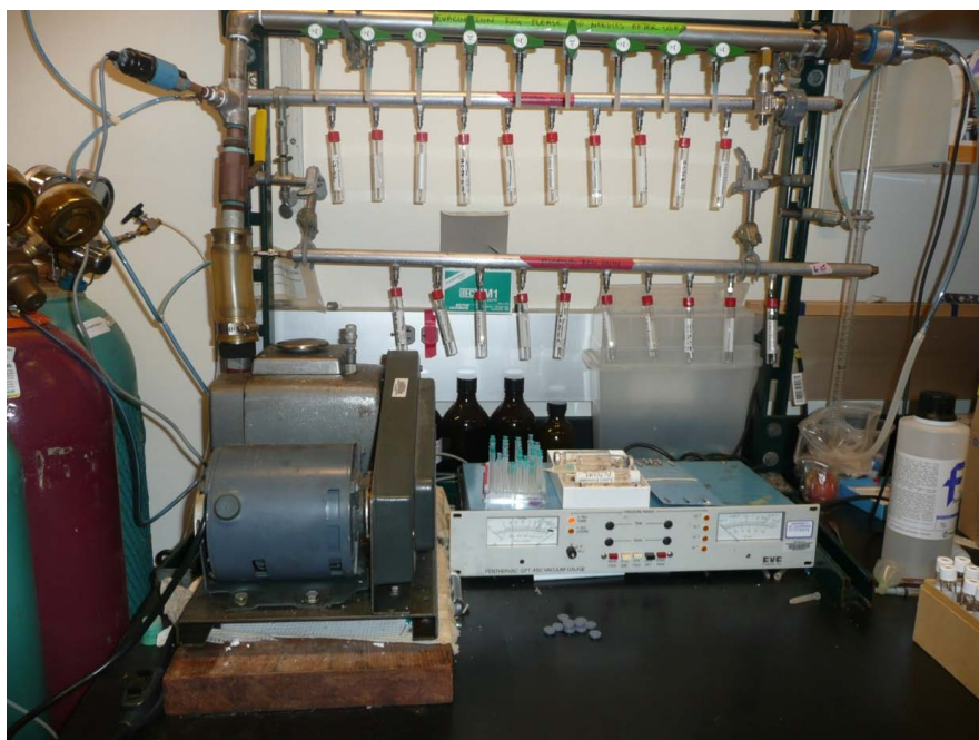
Figure E-1. View of Apparatus Used to Evacuate Vials.
