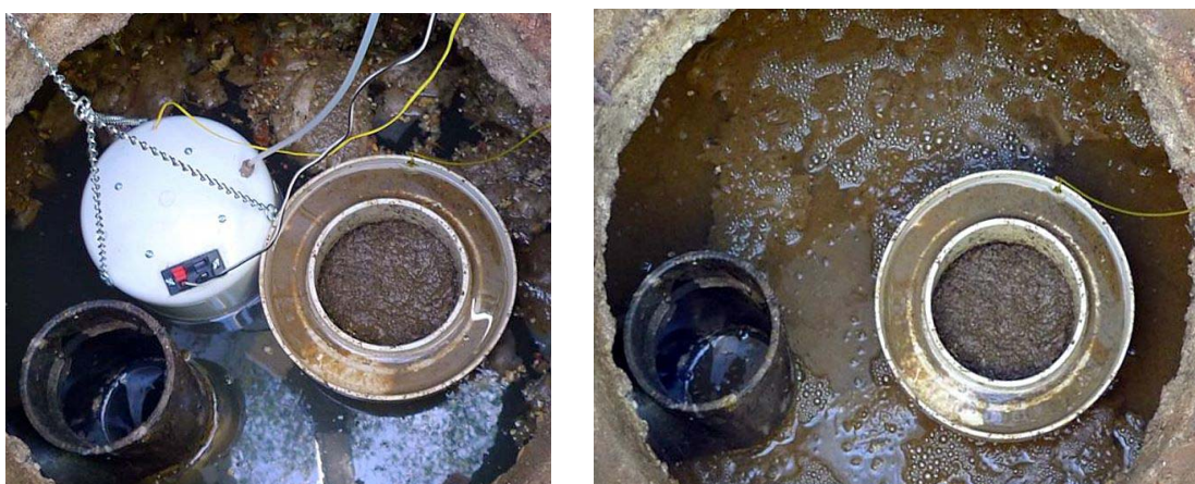
Figure 5-10. Views of Tank at Site 1 (a) Just Before and (b) During a Turnover Event.
