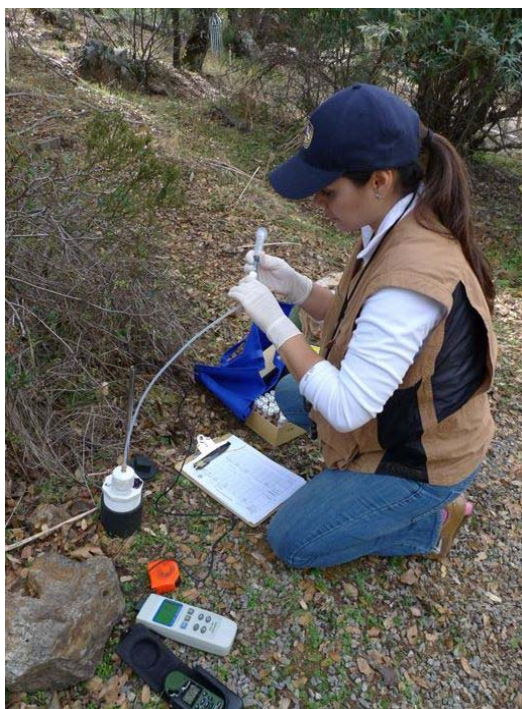
Figure 3-8. Sampling of Gases from the Venting System.
