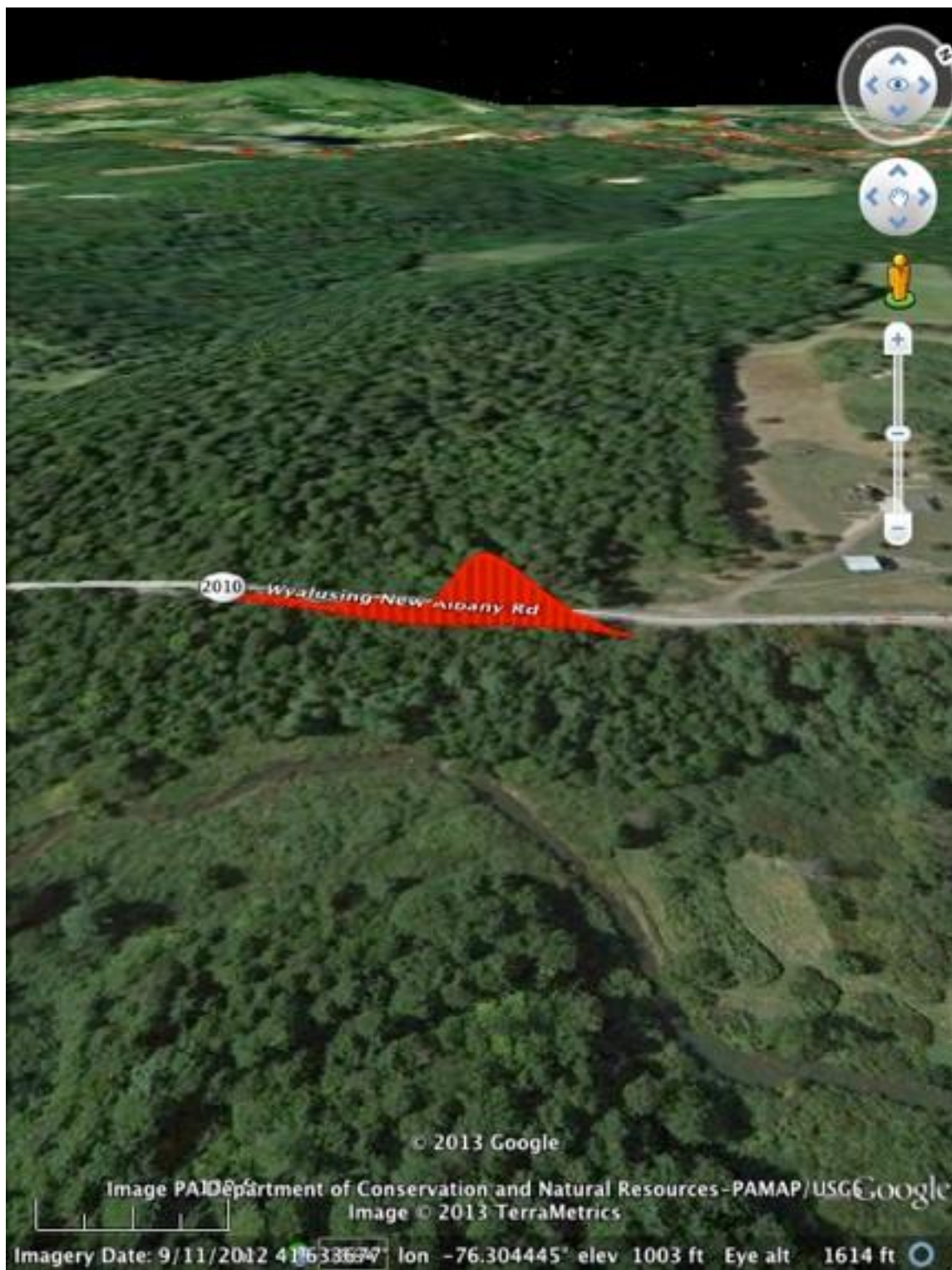
Figure 4. An elevated methane level as rendered by processing of the Wyalusing 31 January 2013 methane survey data to remove values < 1.9 ppm and multiply remainder by 100. Compare to same elevated methane location in Figure 3.
