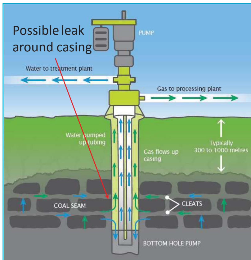
Figure 4.12. Schematic representation of a CSG well showing a possible route for CH 4 leaking outside a casing.
