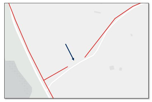
CIE\_B127-B19\_1727589 is a seven-foot long segment that does not correspond to a full span of primary conductor.
