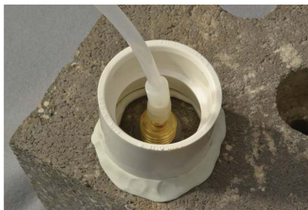
Figure 6. Water dam used for leak detection.
