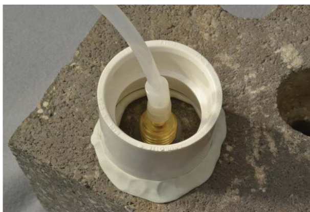
Figure 6. Water dam used for leak detection.
