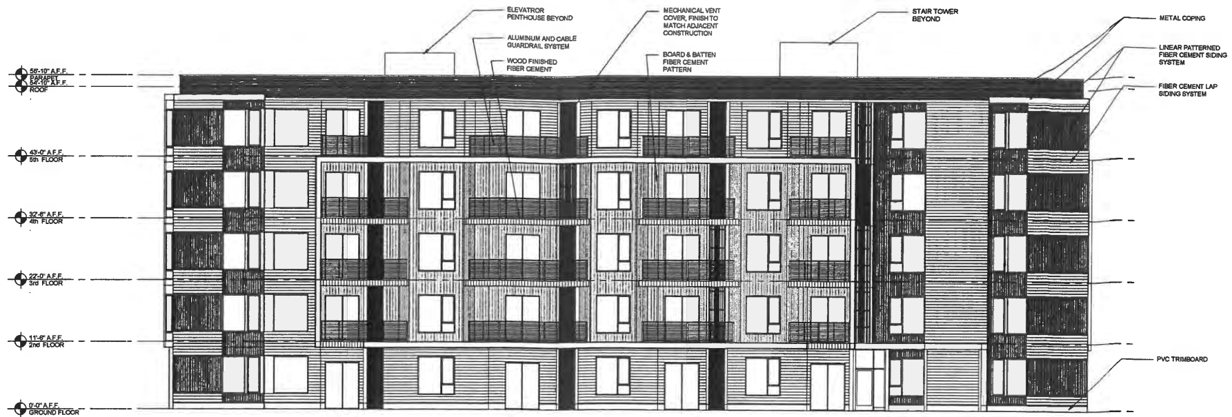
3 NORTH ELEVATION SCALE: 1/8" = 1'-0" BUILDING A SOUTH ELEVATION AND BUILDING B EAST AND WEST ELEVATION SIMILAR. NORTH ELEVATION NOTED FOR TYPICAL MATERIALS USED ON ALL ELEVATIONS.
