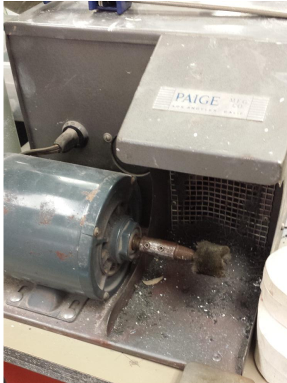
55. Technology Building Kiln Room – Buffing wheel creating dust and debris in room.
