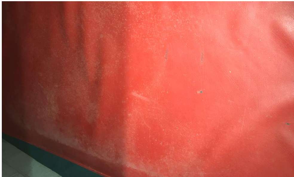
44. Small Gym Wrestling Mat Storage Locker – Fungal growth on stored wrestling mats.
