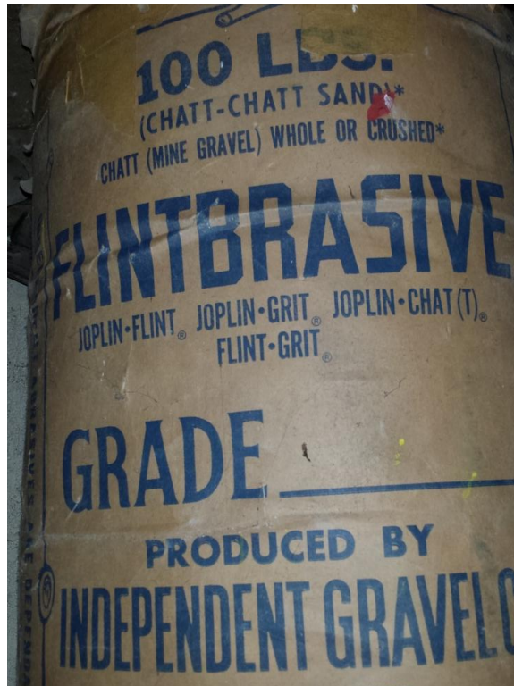
52. Technology Building – Bag of asbestos-containing abrasive in mechanical attic.
