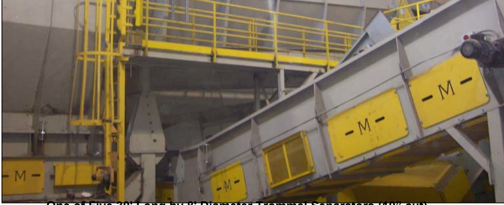
One of Five 30' Long by 8' Diameter Trommel Separators (10" cut)
