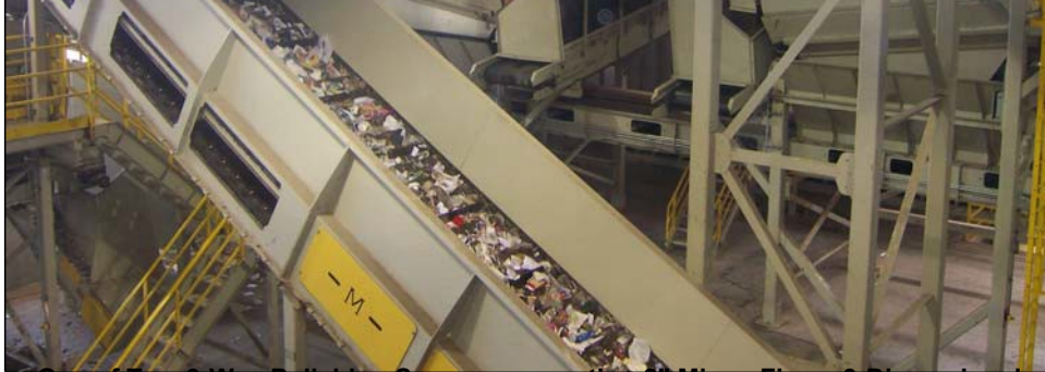
One of Two 3-Way Polishing Screens separating 2" Minus Fines, 3-Dimensional Items (Containers), and 2-Dimensional Items (Paper and Plastic Film). Screen in Back of Photo.
