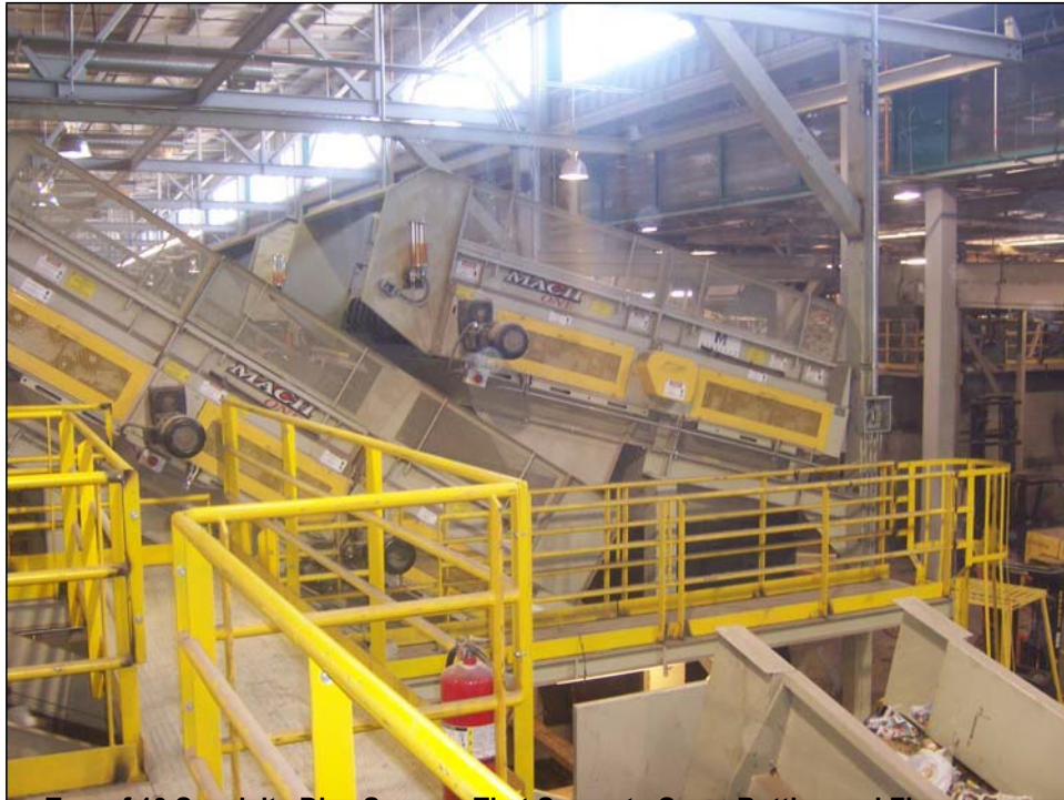
Two of 10 Specialty Disc Screens That Separate Cans, Bottles and Fines From Large Paper
