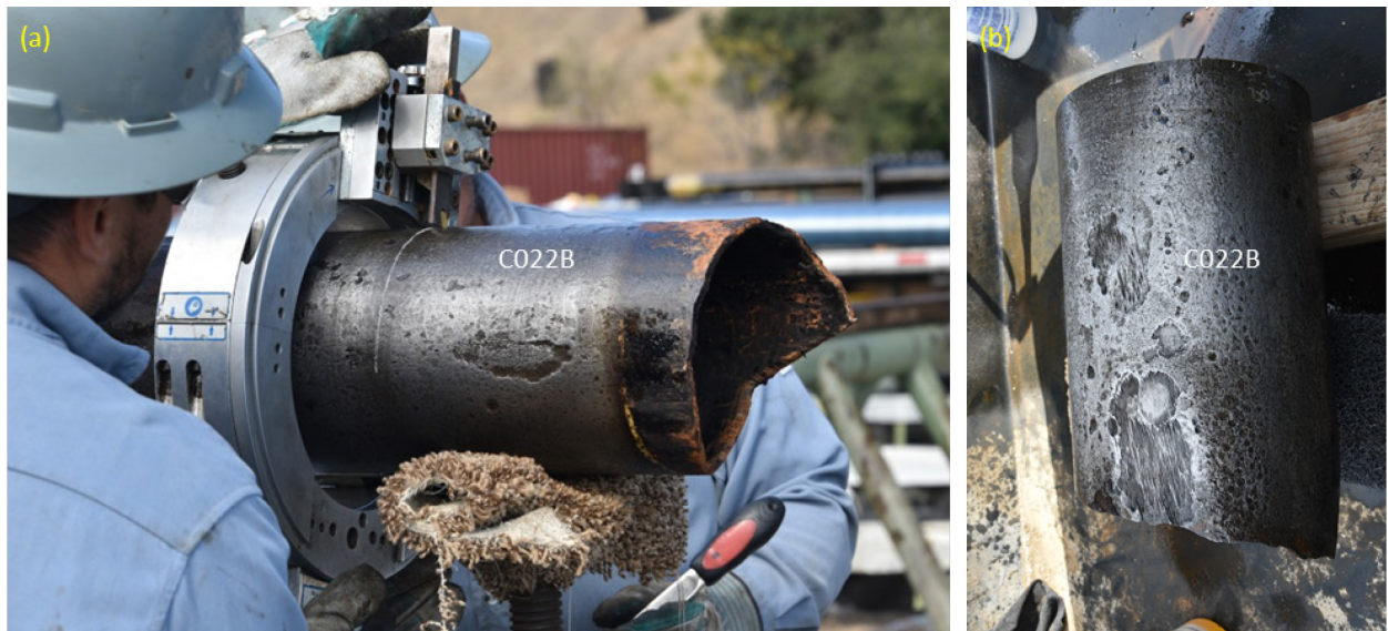
Figure 34: Parted Casing (a) Cutting from C022 and (b) After Cleaning with Sentinel 909
