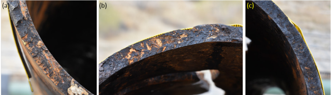
Figure 41: Circumferential Parting Fracture Surface (a) Features, (b) Chevron Marks, and (c) Surface Erosion
