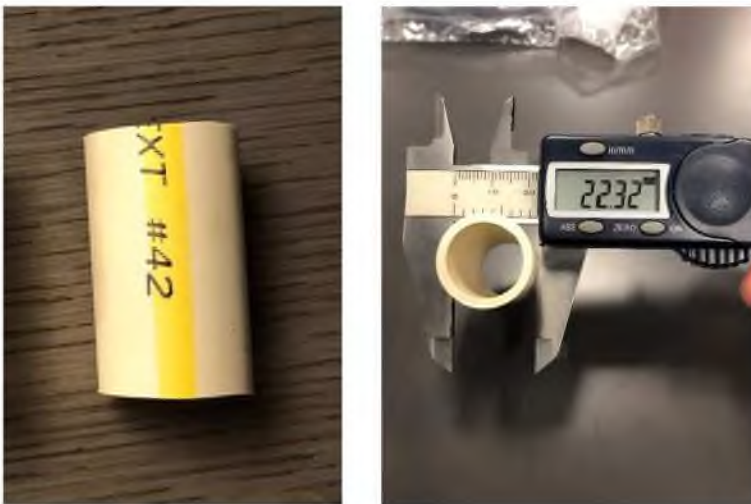
IMAGE 12 - \frac{3}{4} CPVC pipe cut to 4 cm
