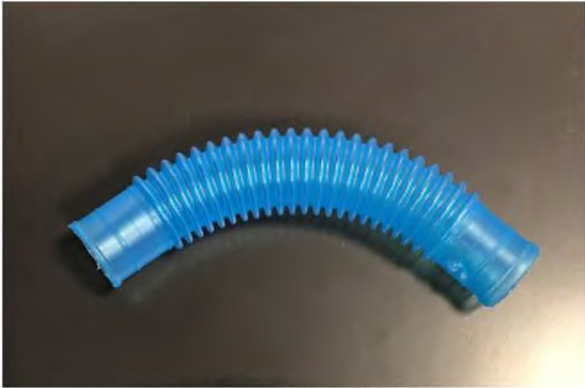
IMAGE 9 - Cut piece of standard large bore tubing
