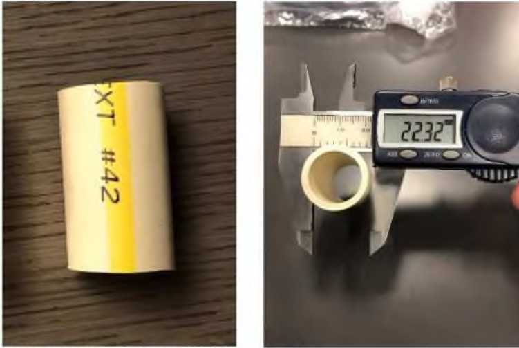
IMAGE 12 - \frac{3}{4} CPVC pipe cut to 4 cm
