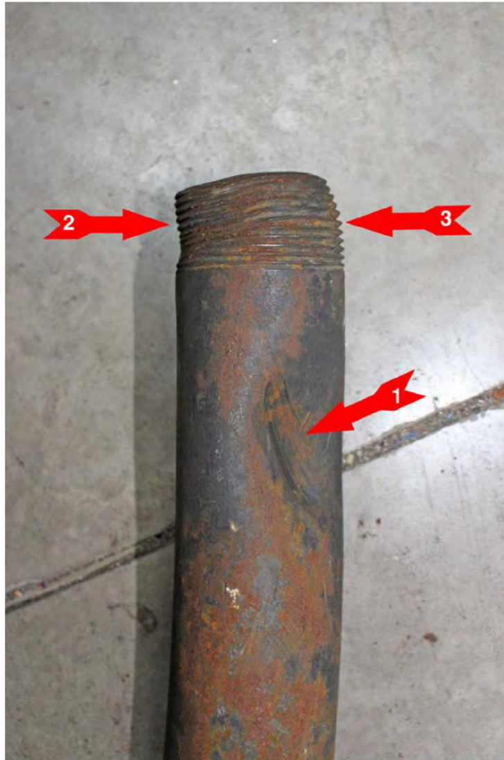
Figure 2 Threaded end of header Arrow 1 Impact location Arrow 2 Compressive bending at threads Arrow 3 Tensile bending at threads
