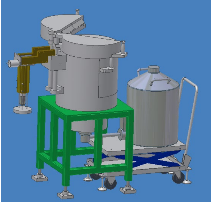
Figure 6. Gross-radiation monitor and spectrometer detector for one AGR-5/6/7 sweep gas line.
