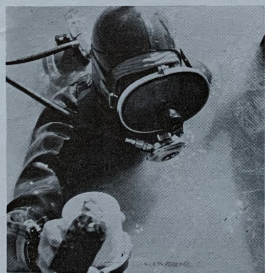
Research diver brings up an underwater thermograph, which records water temperatures near power plant locations.
