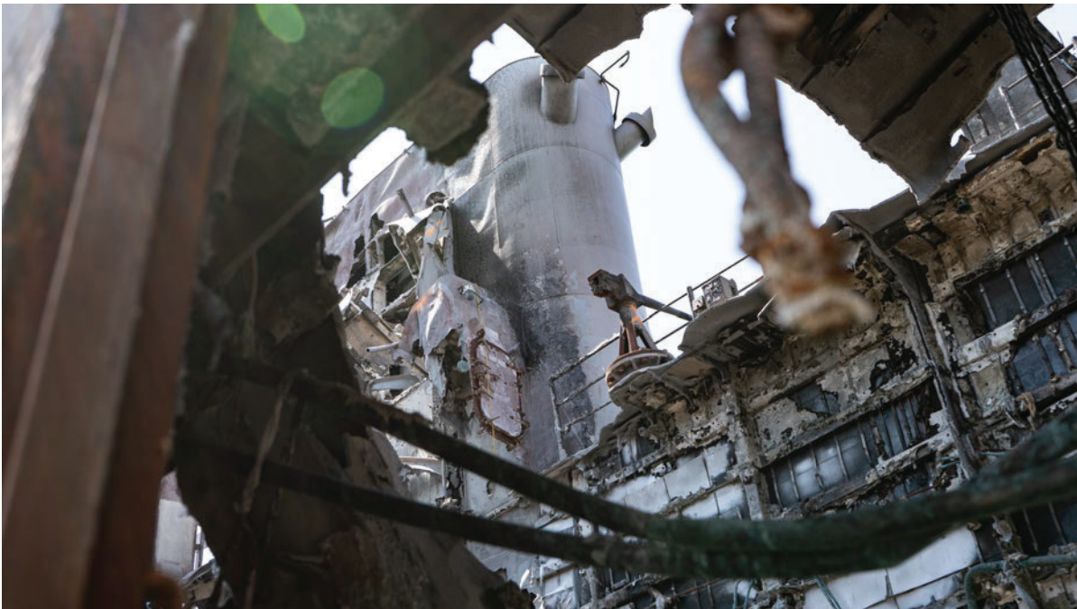
Figure 43 shows the island's interior, illustrating that the overhead has completely burned away.
