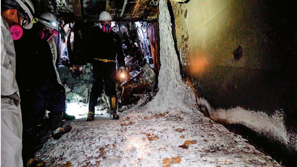
Figure 42 shows investigation team members examining a solidified aluminum flow.
