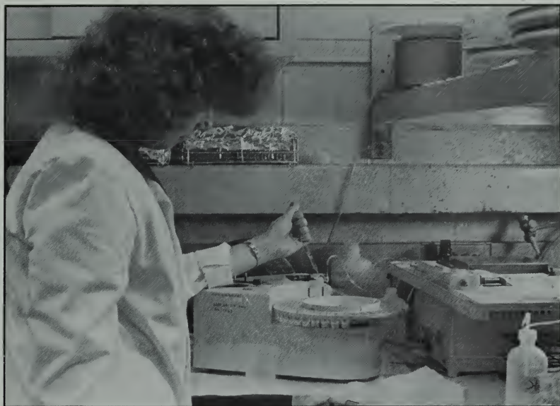
Medical technician uses an automated chemistry analyser for samples used in tricothecene research program at USAMRIID.
