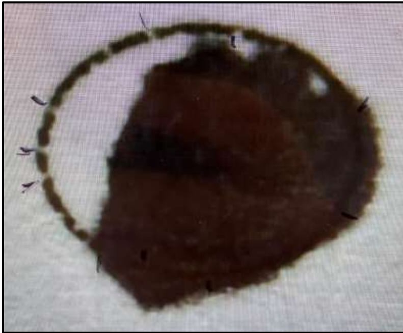
Figure 5 – Example 3 Oval with Anomalous Breaks in the Lines. Anomalous breaks are marked with a pen.
