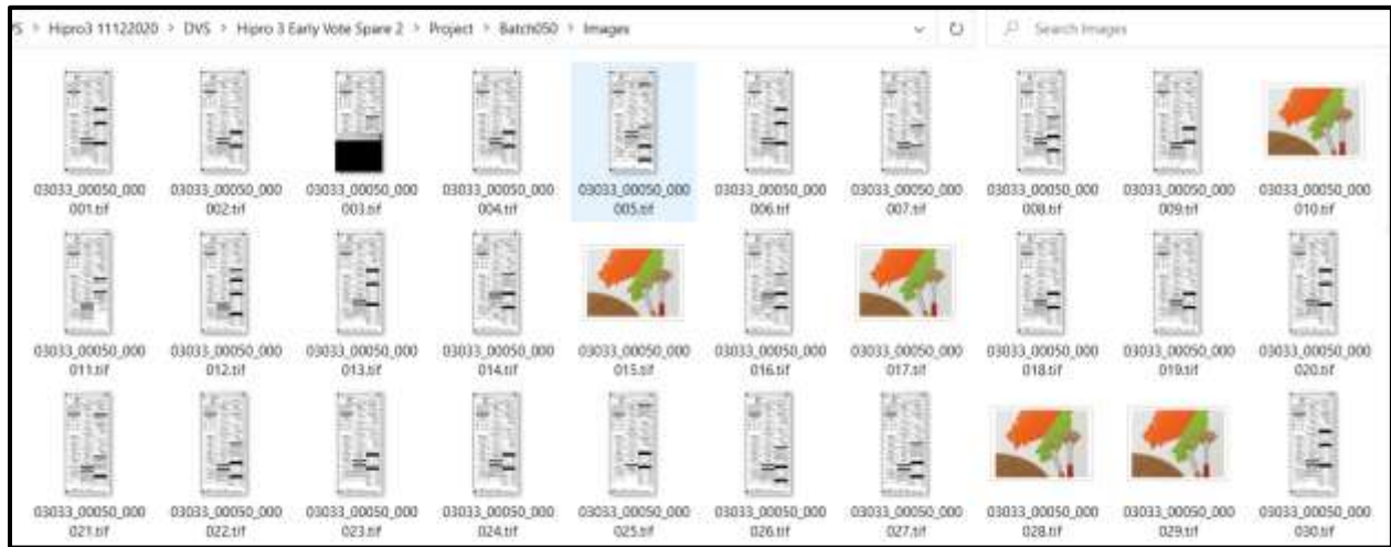
Figure 13 - Example folder showing corrupt TIFF images. The corrupt images either will not display a pre-view at all, or the ballot will be partially blacked out.
