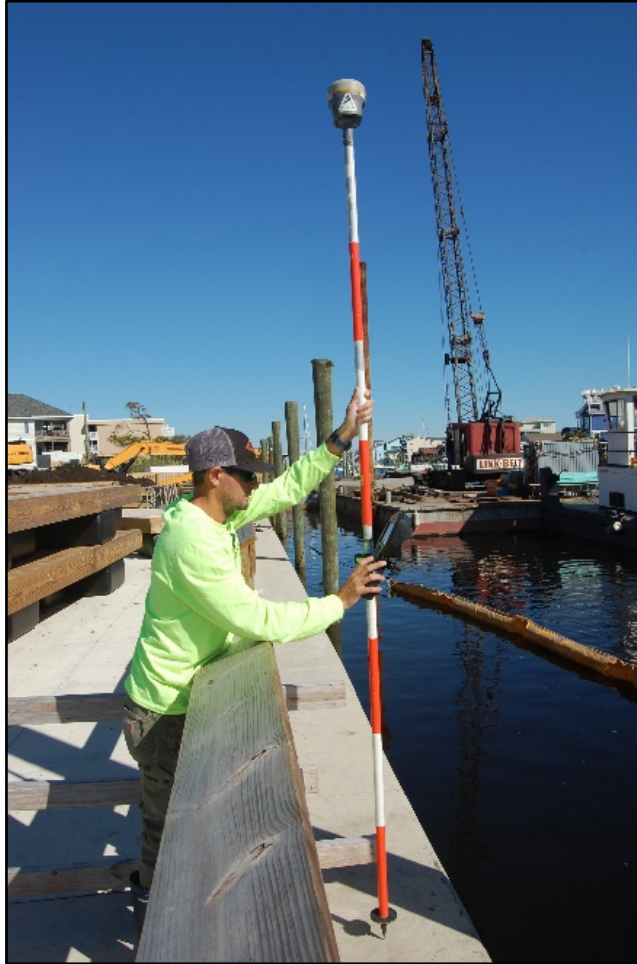
Figure 13. APTIM Conducting Survey of the Bulkheads along the Carolina Beach Yacht Basin.
