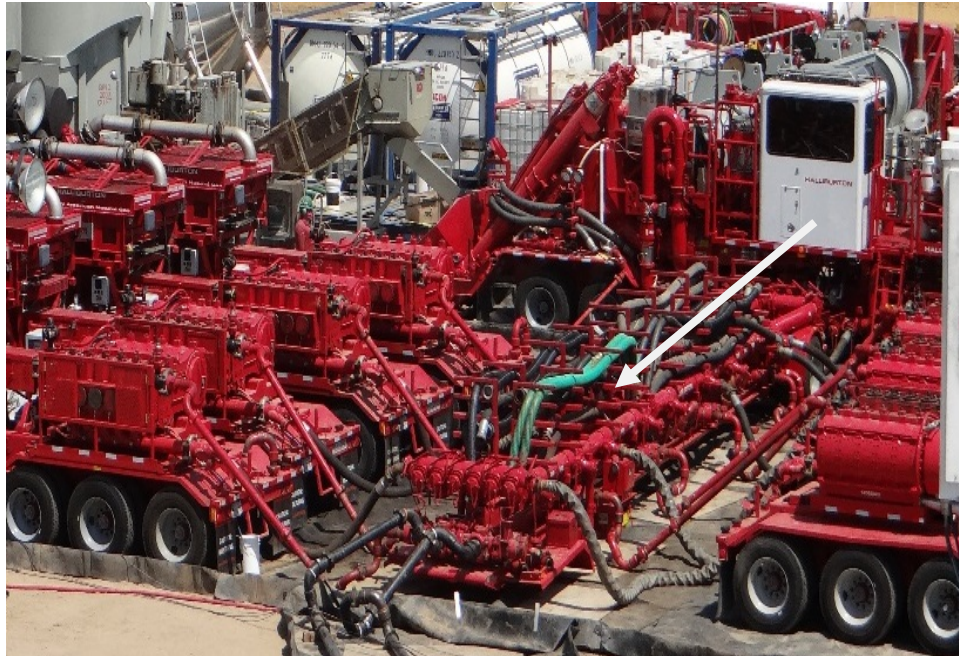
Figure 5-9. Manifold (pointed to by the white arrow).
