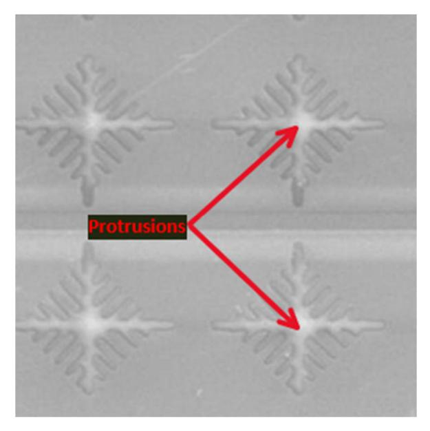
24. The protrusions are positioned at a centralized location between the corresponding pixel electrodes.
