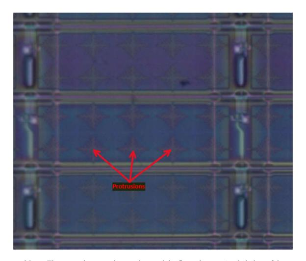
25. The protrusions are elongated toward the first substrate. Angled view of the second substrate showing the protrusions extending from the surface which faces the first substrate when the Accused instrumentality is assembled:
