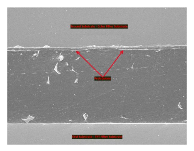
26. The Accused instrumentality includes an alignment layer formed between the protrusions and the first substrate.
