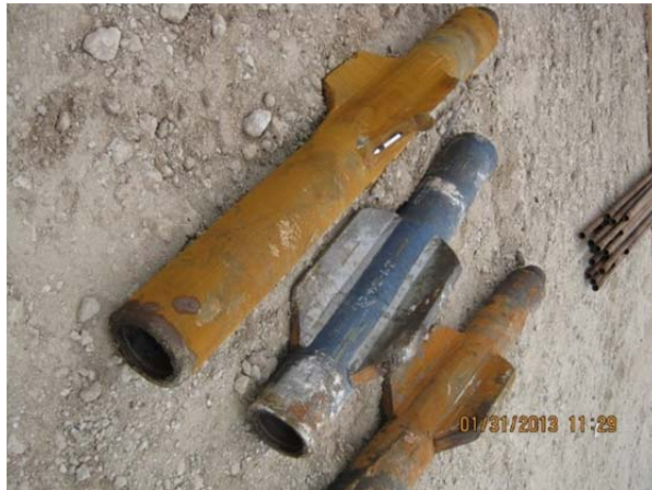
Figure 5: FDEP Photo Indicating Damage to Stabilizer
