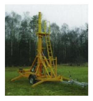
Fast installation of mast systems is often indispensable. According to customer's requirements our systems can be mounted onto vehicles or used in open space. They are available in light, medium and heavy duty versions depending on their height and weight of the object to be fixed, e.g. camera, illumination devices, antenna etc. Out of our range of more than 30 different mast systems we have selected 3 versions. Please ask for a detailed quotation that are sutiable for military purposes as well.
