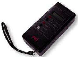
different density then a full one. It also detects radioactive materials. The PKI Contraband Detector directs a beam of energy into the inspected object. A filled space reflects back more energy than an empty space. As PKI
