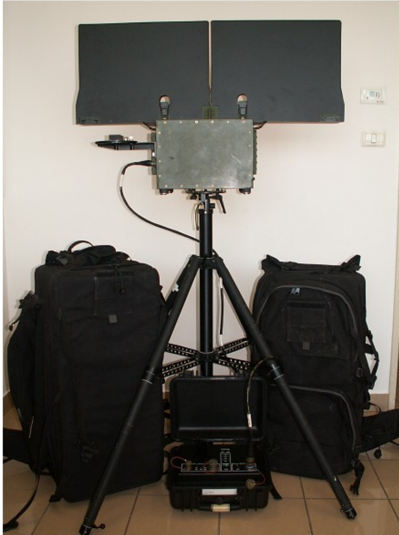
Fully Portable DF System for Fully passive system
