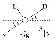
Fig. 1: Forces acting on a skydiver. The solid lines indicate forces while the dotted lines indicate the skydiver's direction of motion and the horizon. **L**, **D** and  $m\mathbf{g}$  are the lift, drag and gravitational forces respectively, where m is the mass of the skydiver and  $\mathbf{g} = 9.81 \,\mathrm{ms}^{-2}$  is acceleration due to gravity. The skydiver is travelling at an angle  $\theta$  to the horizon.
