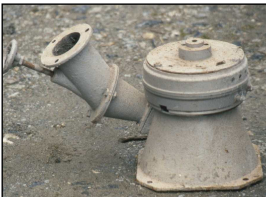
Fig. 7: Chinese-made 100W “family hydro” turgo turbine in use in Vietnam Source: Oliver Paish
