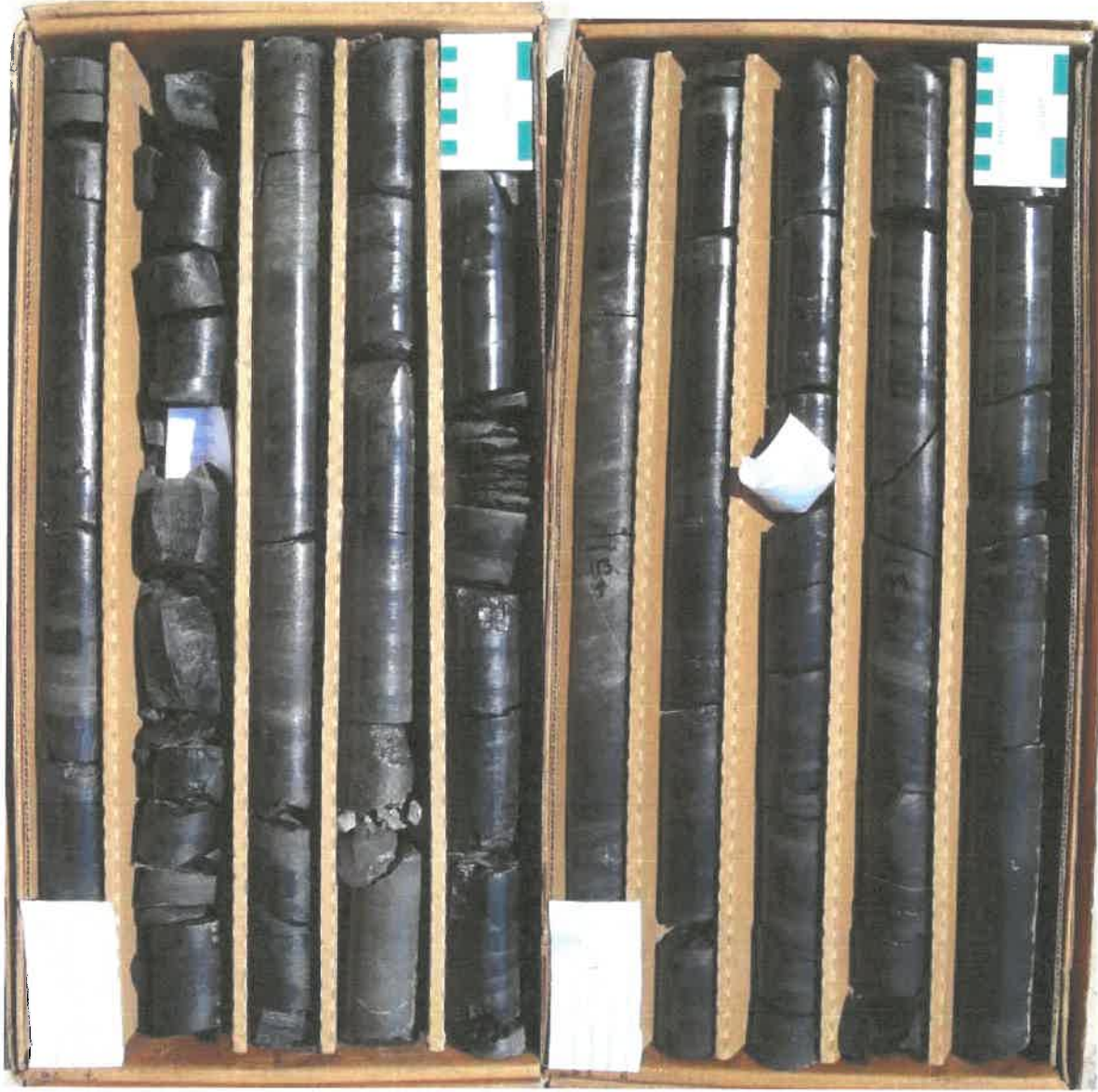
Figure 7. Example drill core from an existing drill core hole (SO-C-2-81 – see previous figure). This shows the diameter of the hole that will be produced during coring.
