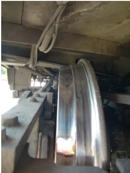
Figure 3 - Trolley #453 Abnormal wear on left side tread. The narrow flange and uneven tread surface requires the wheel to be trued.
