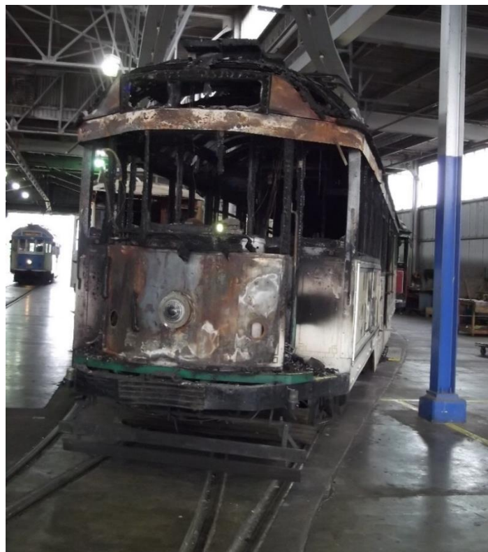
Figure 13 – Trolley #553 showing the burnt out shell at one end of the car.
