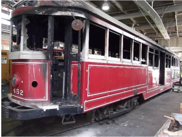
Figure 7 – Trolley #452 after the fire
