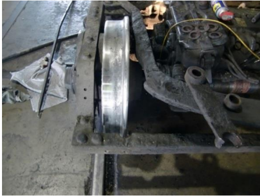
Figure 2 - Wheel with normal wear
