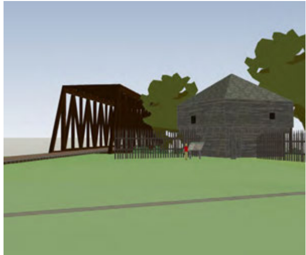
Model view showing the proposed 8' high stockade fence segments on the original fence footprint.
